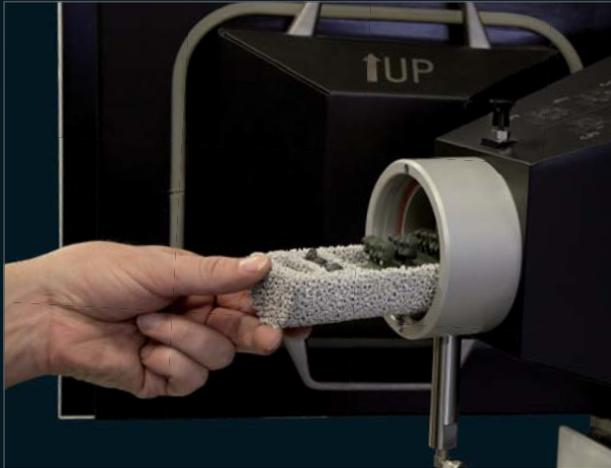
*Combustion chamber Zirkonofen 700 Ultra-Vakuum sintering furnace for up to 120 zirconia and 25 sinter metal elements*
