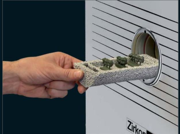
*Combustion chamber Sinterofen 300S sintering furnace for approx. 50 Sintermetall elements; 2 full arch bridges or 6 bars in one process*
